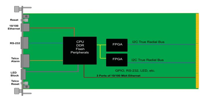
FIGURE 2. VT019 Functional Block Diagram
